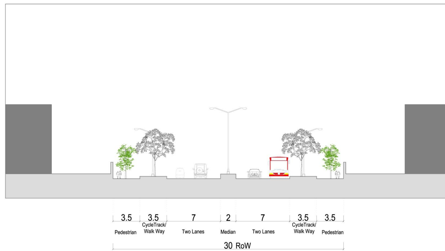
3-16, 30 mt. Row, Road Section
