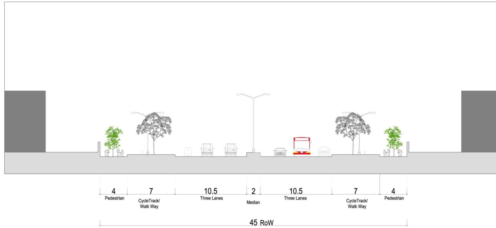
3-15, 45 mt. Row, Road Section
