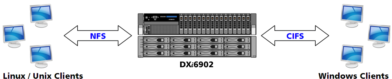
Figure 12: NAS Backup using CIFS/SMB and NFS
