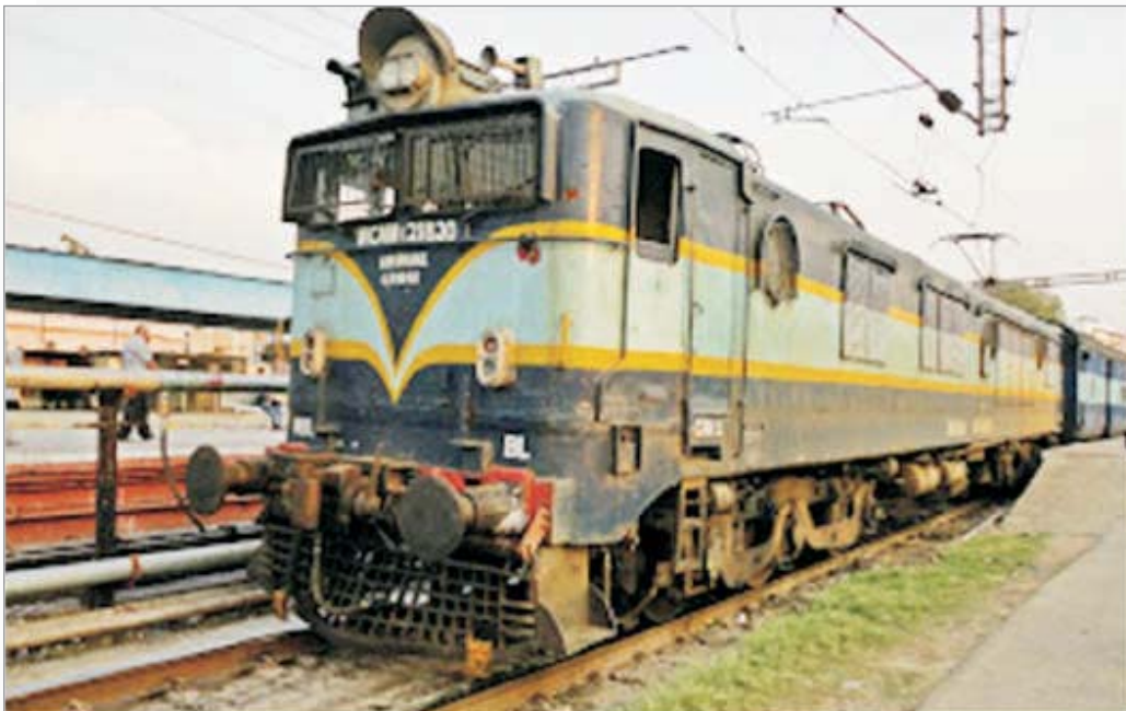
WCM 1 (AC/DC) - Introduced in 1975 having hp of 2930 DC/3640 AC & max. speed 110 kmph. This class of loco was generally found only in Bombay Central - Ahmedabad section.
