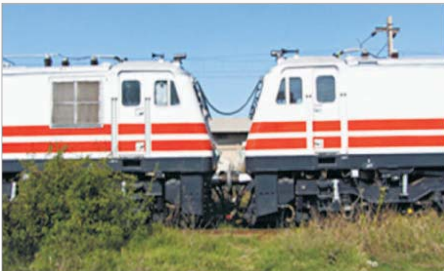
WAP 5 MU with Power through HV Cable
