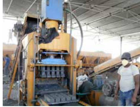
Brick manufacturing machine
