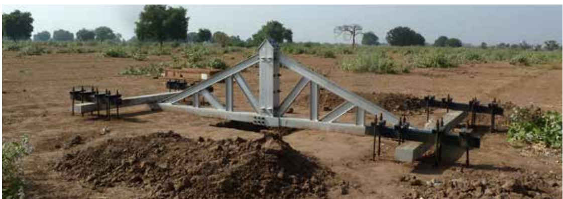
Figure 28. Test setup for geotechnical investigations.
