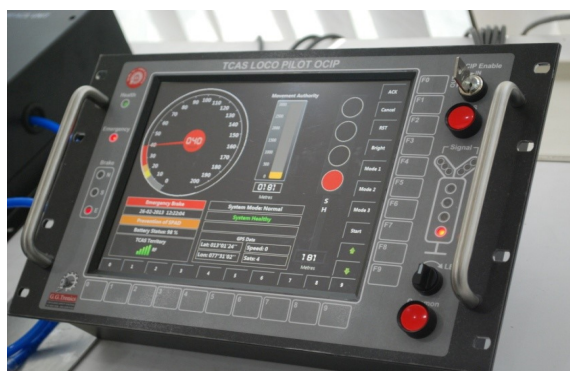
Driver Machine Interface (DMI) of TCAS
