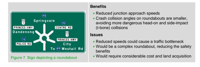
In this approach a roundabout would replace the current junction.
