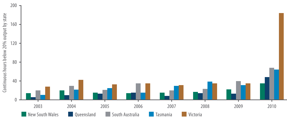
Figure 10: Continuous hours of low wind production where less than 20 per cent of the state’s overall capacity for wind was generated
