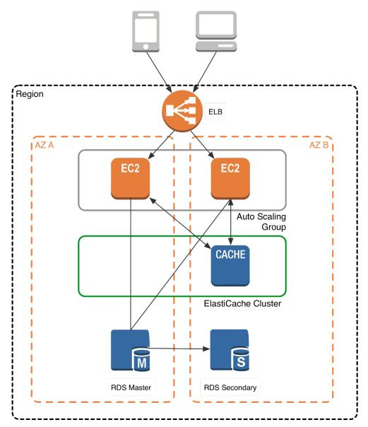
In this architecture diagram, the Amazon EC2 application instances are in an Auto Scaling group, located behind a load balancer using Elastic Load Balancing, which distributes requests among the instances. As requests come into a given EC2 instance, that EC2 instance is responsible for communicating with
