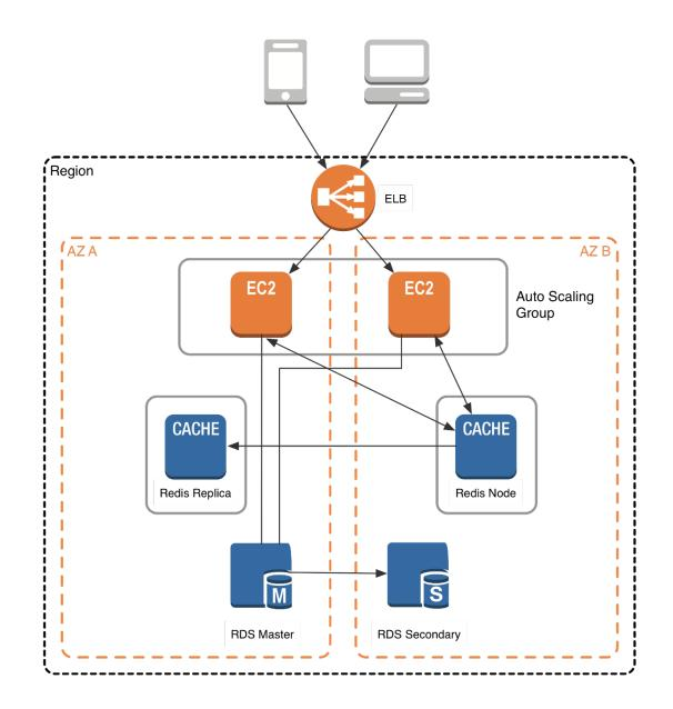
ElastiCache for Redis has the concept of a primary endpoint, which is a DNS name that always points to the current Redis primary node. If a failover event occurs, the DNS entry will be updated to point to the new Redis primary node. To take advantage of this functionality, make sure to configure your Redis client so that it uses the primary endpoint DNS name to access your Redis cluster.
