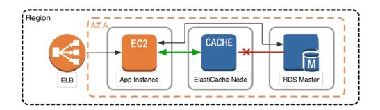
To keep your cache nodes as secure as possible, only allow access to your cache cluster from your application tier, as shown preceding. ElastiCache does not need connectivity to or from your database tier, because your database does not directly interact with ElastiCache. Only application instances that are making calls to your cache cluster need connectivity to it.
