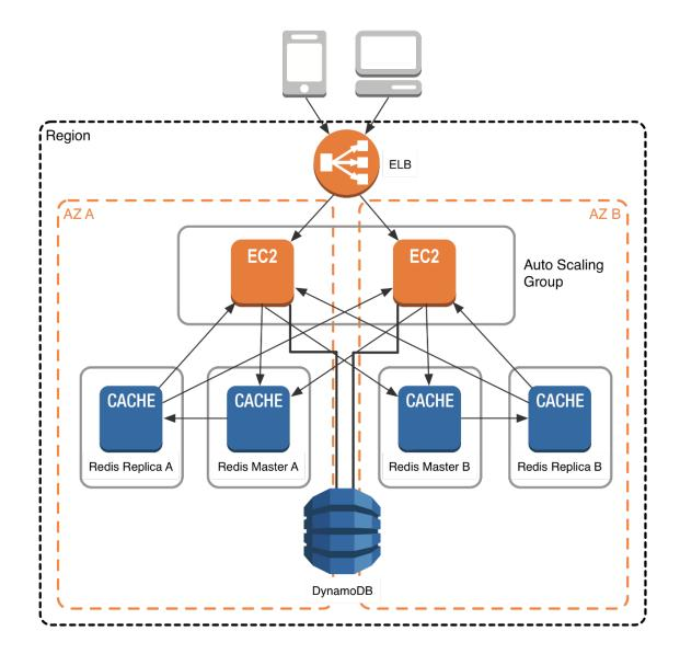
For the purpose of simplification, the preceding diagram shows replicas in the same Availability Zone as the primary node. In practice, you should place the replicas in a different Availability Zone. From an application perspective, continuing with our Java example, you configure two Redis connection pools as follows:
