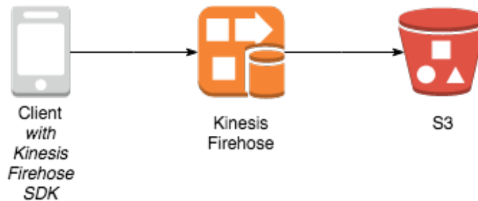
Figure 12: Reducing cost of sending data to Amazon S3 by streaming directly using the Kinesis Firehose SDK
