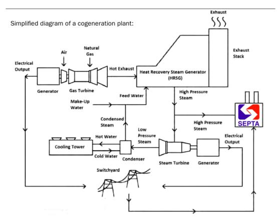
energy are interrupted. This causes cogeneration plants to have far less control of start-ups or shutdowns as compared to a plant generating only electricity. Also, it limits the opportunities for many cogeneration plants to either increase or decrease their energy generation, which can be significant in cyclical demand fluctuations that occur with the seasons. Additionally, as an industry insider said at a conference last year, it "is not that much more efficient."
