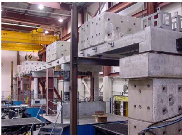
Figure 12. Model bridge tested at the University of Nevada, Reno, NEES facility. © 2007 by Mehdi Saiidi.
