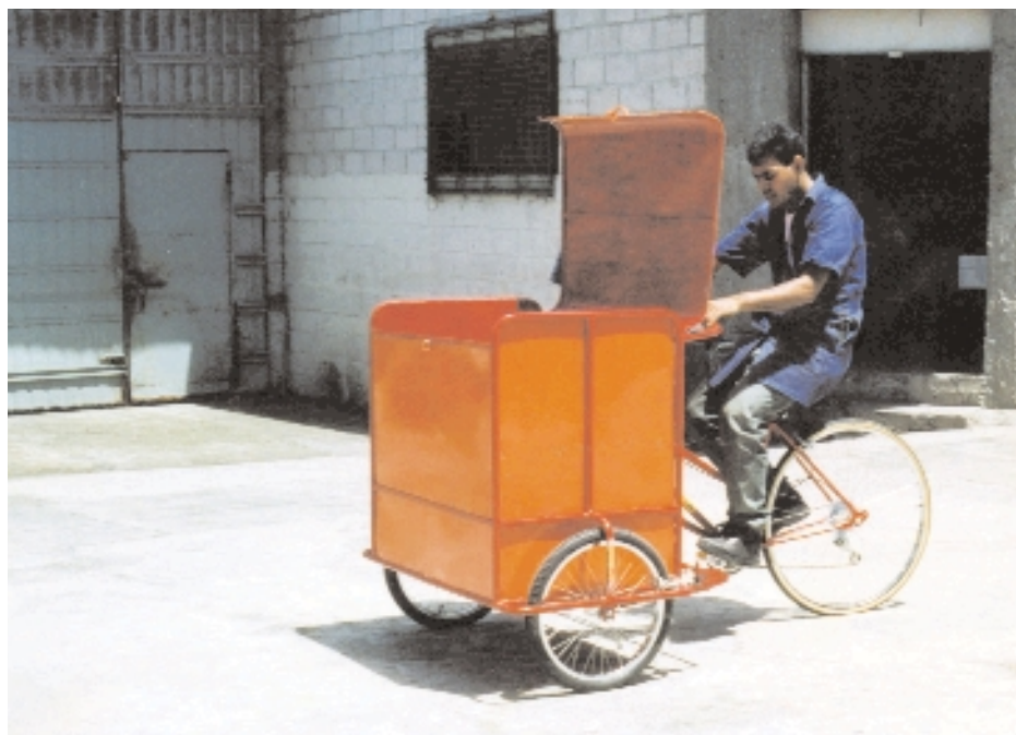
To complement their transport concept, FoE El Salvador designed load carrying tricycles with 18 speeds capable of carrying up to 90 kg.
