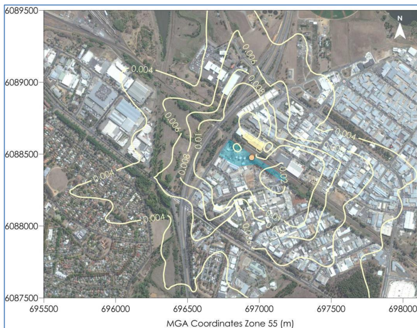
Figure 6: Predicted maximum 1-hour average HCL concentrations ( \mu\text{g}/\text{m}^3 ) – Impact assessment criterion (allowable limit) 140\mu\text{g}/\text{m}^3
