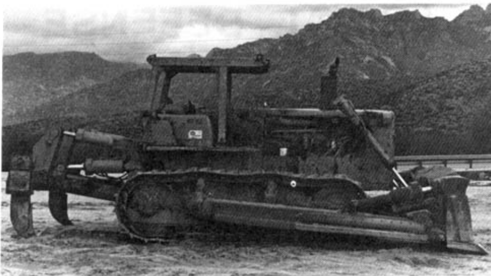
Bulldozer. Note the smoke stack (exhaust pipe).
