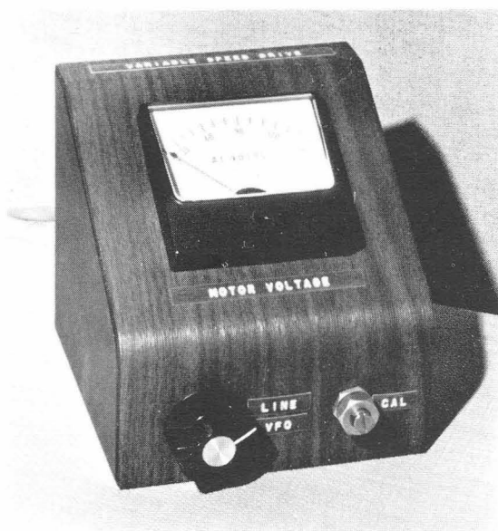
FIG. 1. COMPLETED VFO CONTROL UNIT. OTHER SCHEMES, SUCH AS RACK PANEL MOUNTING, ARE POSSIBLE.
