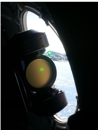
View from the source aircraft during a data collection flight. The backside of the AFIT Active Pointer Tracker beam steering gimbal mirror is shown as it illuminates the Notre Dame beam steering turret with its green source laser at a distance of 50 meters.
