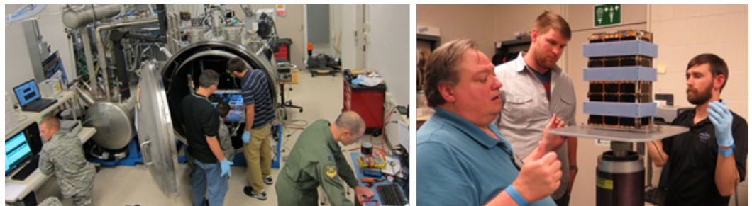
Figure 1. AFIT students and staff prepare a CubeSat for environmental testing (left) and Mr. Jesse Coffee (Pumpkin Inc.) observes AFIT research assistants Mr. Phil Smith and Mr. Chris Sheffield measuring the mass properties of a SUPERNOVA spacecraft (right).
