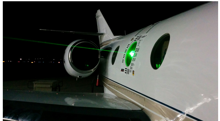
Ground testing and alignment of the AFIT pointer tracker 2.5 Watt green laser to the Notre Dame AAOL turret at a distance of 150 meters.
