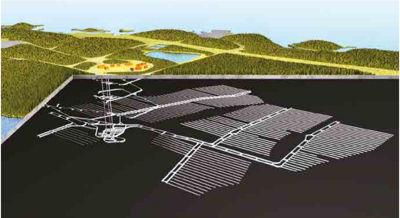
Figure 6: An illustration of Posiva's repository for the disposal of spent nuclear fuel at Olkiluoto, western Finland. Image courtesy of Posiva Oy.
