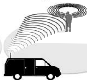
2. The stingray system, which mimics a cellphone tower, gets the target phone to connect to it.
