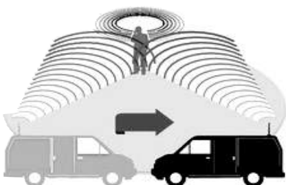
4. The vehicle can then move to another location and again measure the phone's signal strength.
