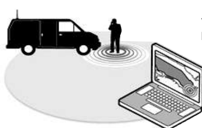
5. By collecting signal strength in several locations, the system can triangulate and map a phone's location.
