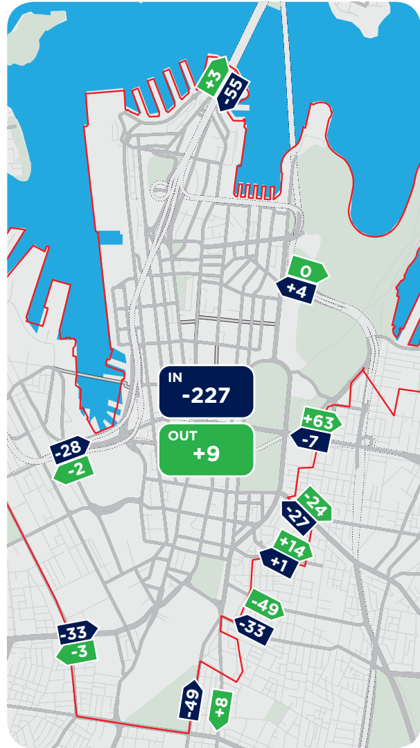
Figure 4.62 Light rail and redesigned bus network am peak hour (8:00 to 9:00am) change in bus volumes
