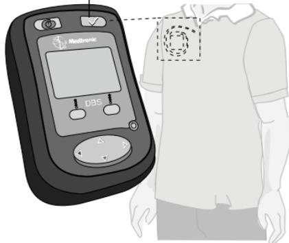
**Figure 2.7** Press the **Check** key to synchronize your neurostimulator and patient programmer.
