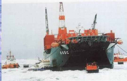
Single Steel Drilling Caisson (note co-author Wim Jolles standing on anchor buoy to the right in red survival suit)
