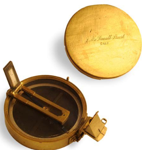
Prismatic compass owned by John McDouall Stuart and used on his successful crossing of Australia in 1862.
