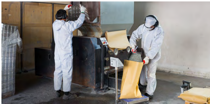
Component packaging trays are shredded and sent to another plant to be recycled.
