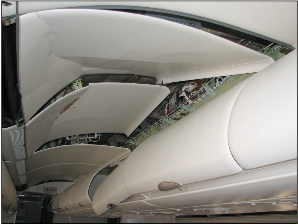
Figure 50: Example of damage to the ceiling panels in the aisle (rear section)
