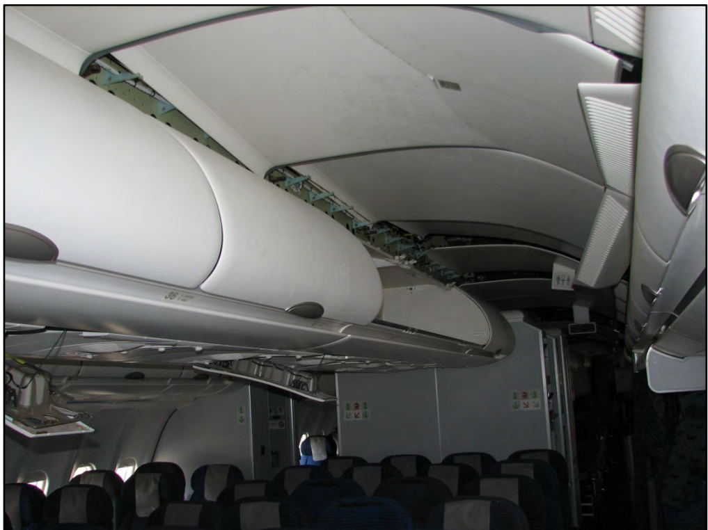
Figure 51: Example of damage to the ceiling panels in the aisle (centre section)
