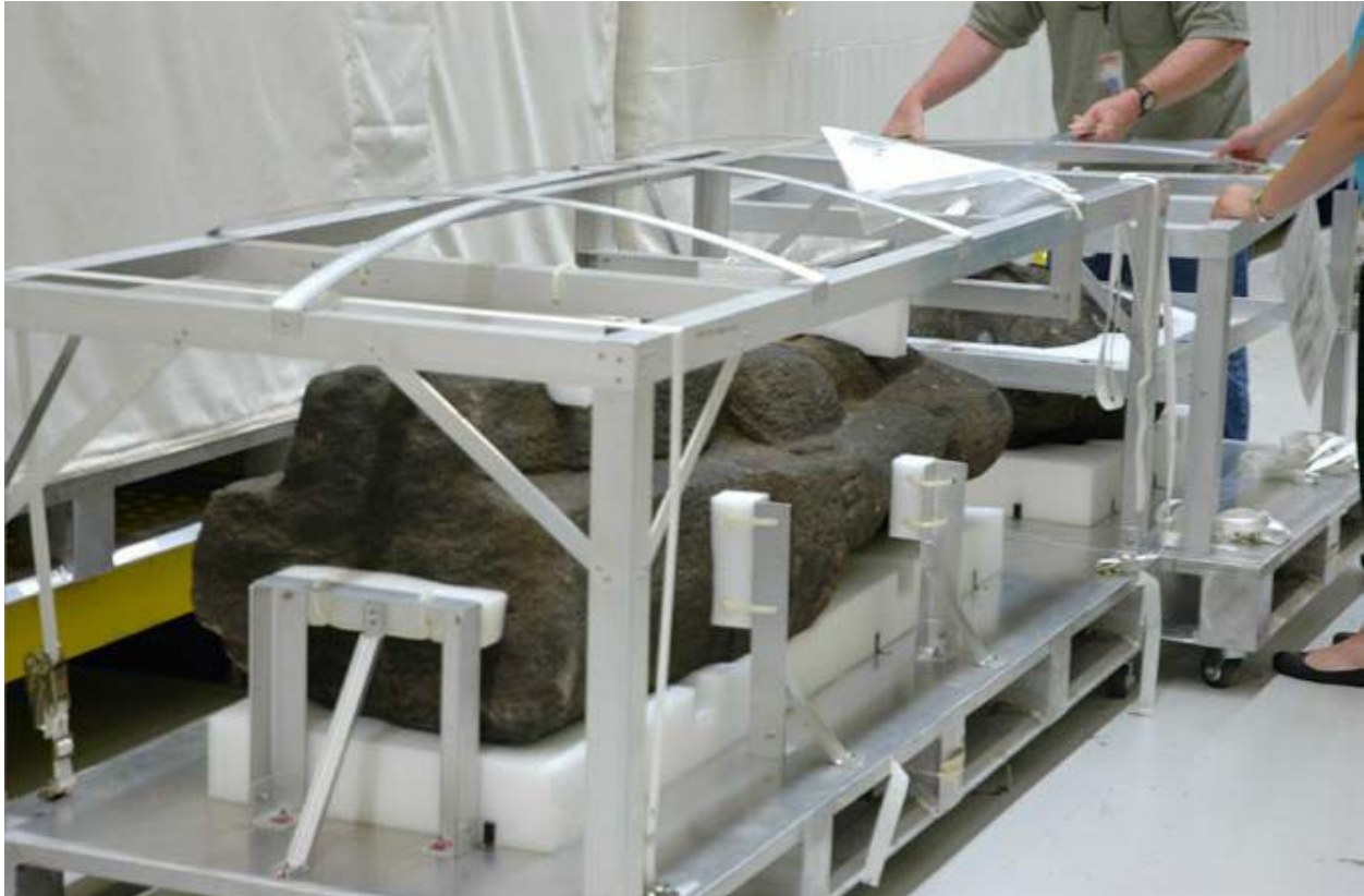
Torso and head pallets for the female figure with metal supports in place.
