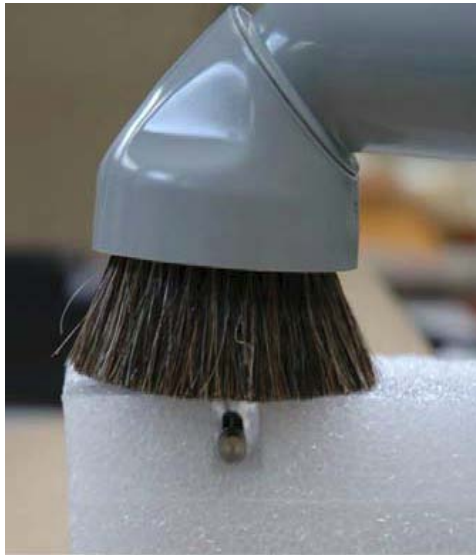
Setup measuring normal forces on a simulated textile surface with the manometer.
