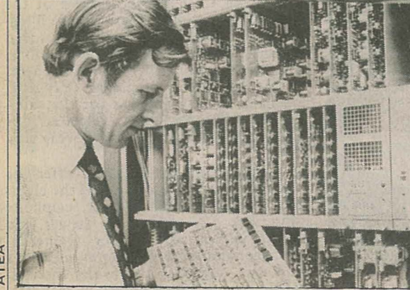
AXE exchange: replaced Step by Step, and all new exchanges introduced since 1980 have been this fully computerised exchange. An average exchange would employ only 0.5 people if Telecom's proposal for centralising control of exchanges goes ahead.
