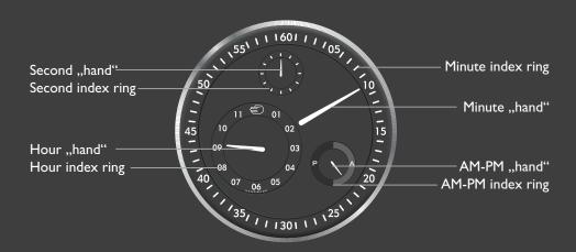
The time is displayed by a flush mounted revolving dial that embodies all the graphical elements in one plane 0.2mm under the 3D shaped sapphire glass. The revolving dial plate points out the minutes, the sub-dials inside the main dial plate indicate the hours, seconds and 24h. The sub-dials orbit a virtual axis similar to the moons around Saturn. Graphically, the time seems to be displayed on the outer surface of the watch.
