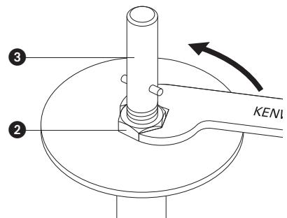
**high temperature flexible beater** - this tool should just touch the bottom of the bowl.
