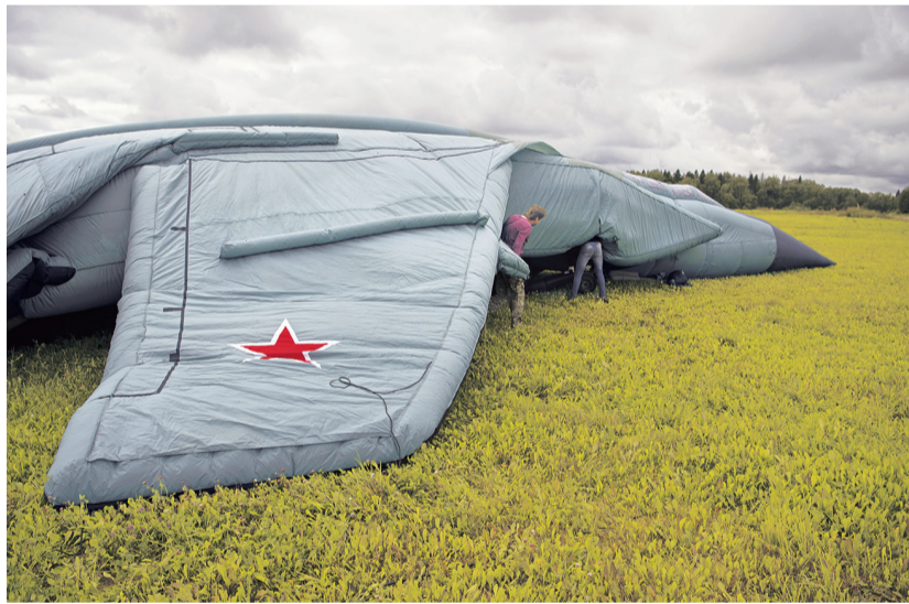
A full-size mock-up of a Russian MIG-31 fighter jet being inflated in a field near Moscow. Many such replicas are manufactured by Rusbal, a hot-air balloon company.
