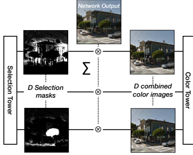
Figure 3: The basic architecture of our network, with selection and color towers. The final output image is produced by element-wise multiplication of the selection and color tower outputs and then computing the sum over the depth planes. Fig. 6 shows the full network details.
