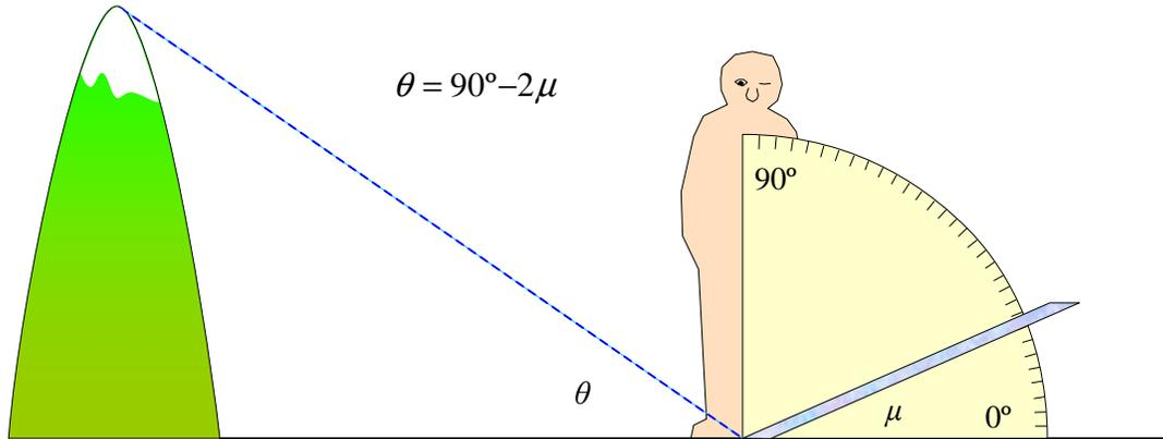
**Figure 8:** Angles must be taken from the ground, for which purpose you might like to tilt a mirror until the reflected mountaintop touches the ground at your feet under the plummet line of sight. Only bear in mind that, because mirrors are whimsical little things, the angle  $\theta$  to the mountaintop is  $90^\circ$  minus twice the tilt  $\mu$  of the mirror.
