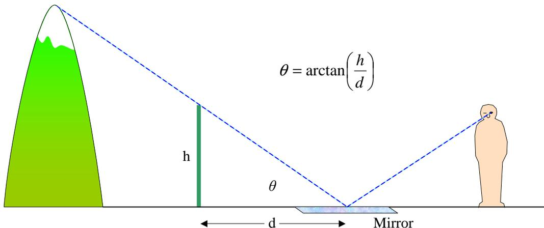
**Figure 9:** An alternative method of finding the angle  $\theta$  from a point on the ground to a hilltop makes use of a mirror on the ground and a stick lined up with the reflected hilltop.<sup>1</sup> This method was first described in Euclid's *Optics* (Proposition 19).
