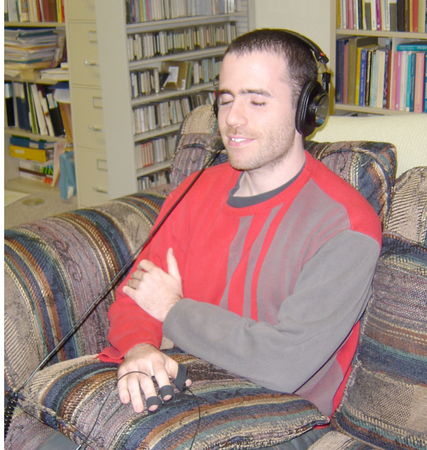
Figure 1: Joshua Penman with GSR electrodes attached to his index and middle finger, and a pulse transducer attached to his thumb.
