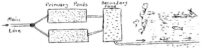
In the primary ponds the refuse will dry out and break up, and the water in the secondary pond will be fairly clean. This water will then run down a 400' long pipe into the sea. A 6' high man-proof fence will go around the ponds, so that may cramp the style of any junior swimmer.
