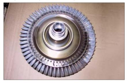
FIGURE 11: LQH left engine compressor turbine assembly
