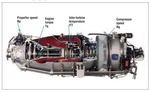
In addition, outside air temperature, indicated airspeed, pressure altitude, engine torque (Tq), and propeller speed (Np) are required to be recorded. The manufacturer's computer software model calculates the predicted values of the three gas path parameters using these other five parameters. The differences between the recorded values and the predicted values of Ng, ITT and Wf are termed 'deltas'.
