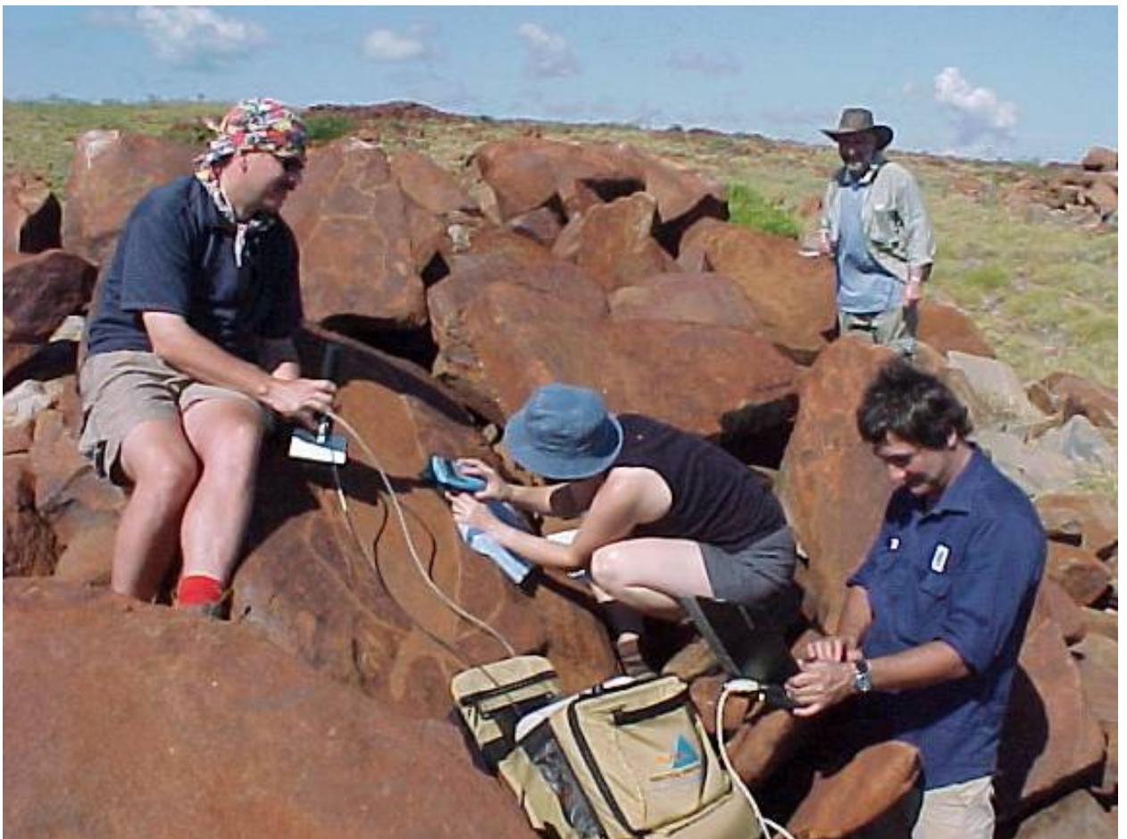
Figure 4. ASD fieldSpec Pro operating on petroglyphs in the Burrup Peninsula
