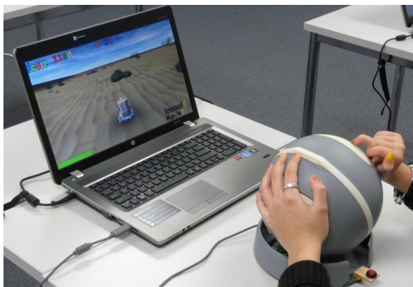
Figure 4: A functional prototype controller being trialled during one of the focus group sessions with children with hand impairments.
