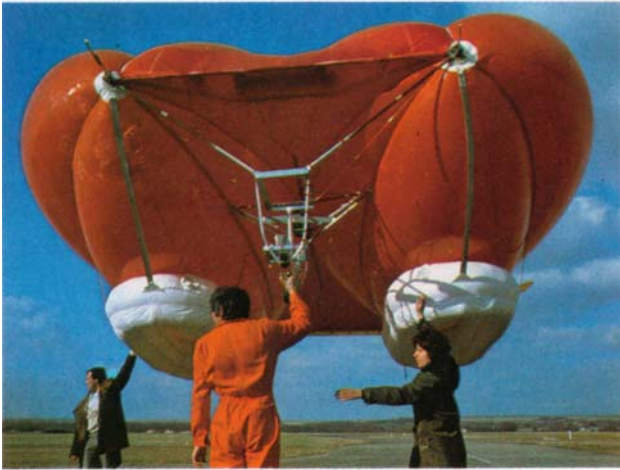
Fig. 15. French double trilobed airship 'Dinosaure'
