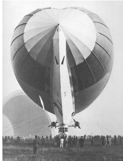
Fig. 21. French Zodiac bi-lobed airship "E-8"
