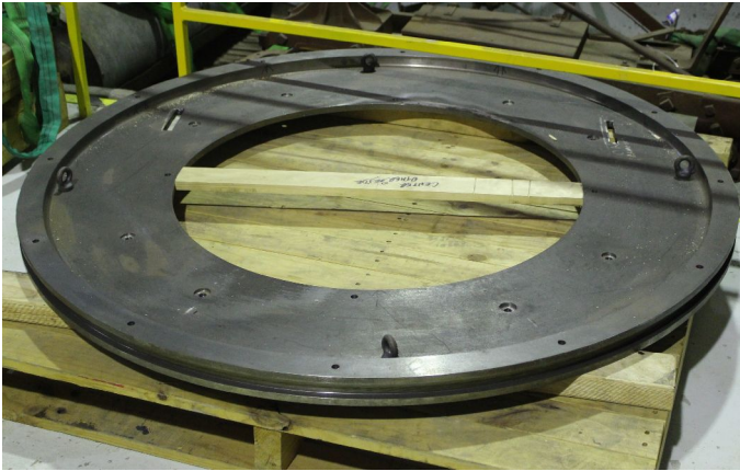
The machined, newly cast Declination Clamp Disk - the original cast-iron broke into five (easy?) pieces long ago
