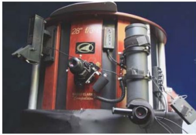
Figure 5. The working end of Barry Clark's 71cm aperture f/3.6 'Compulsion' telescope.
