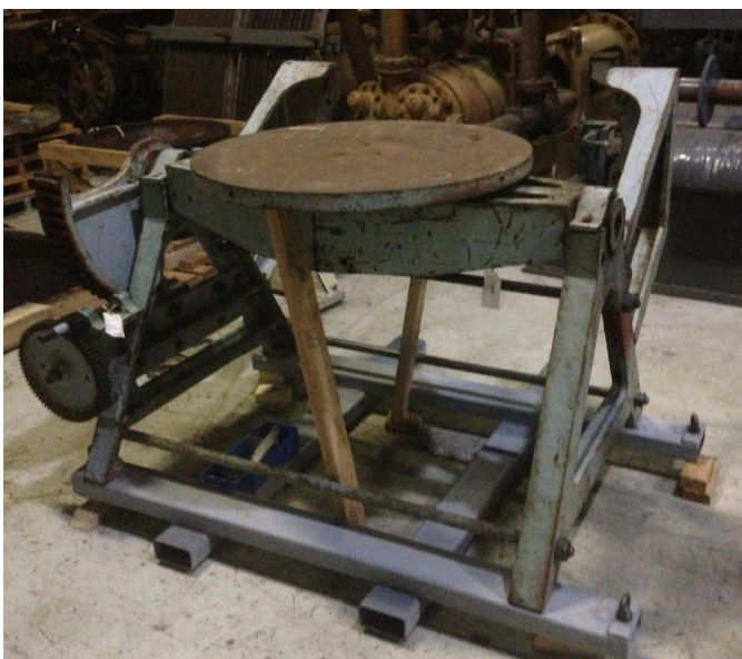
Front view - the circular table upon which the 1300-kg metal mirror sat; it must have been very top-heavy
