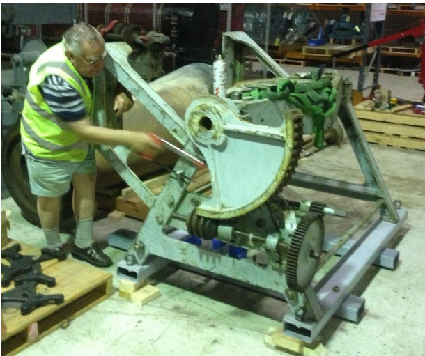
David sawing the end off a specially made steel strut that holds the two sides of the frame together
