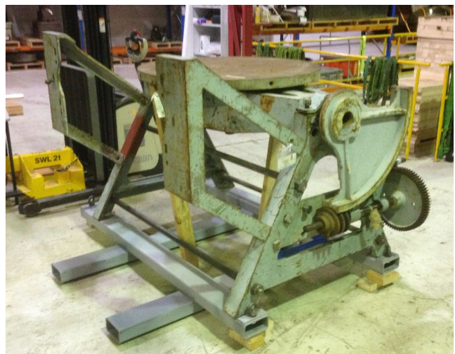
Rear view of the MGPM - the backplate (not yet fitted) attaches to the two vertical areas
