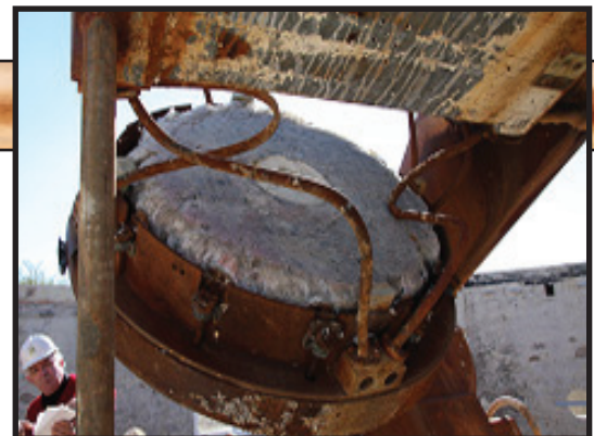
This is the shattered Pyrex mirror, in the original GMT mirror cell– those struts were once straight. And that's Jim Pollock, wondering how we are going to restore it. But we will!
