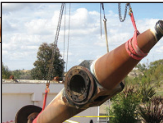
Here's the cubic casting of the polar axis that held the declination axis, starting its journey back home to Melbourne. The upper (southern) conical part is original; the lower conical part was added at Mt Stromlo.
