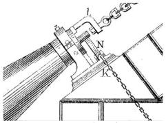
Located at the upper pivot of the polar axis are bearing relief mechanisms controlled by counterweights suspended over the side and the front of the south pier.
