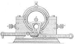
The upper pivot bearing showing the relief mechanism. The central bar is lifted by the cantilevers pulled by suspended weights.
