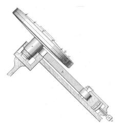
The lower pivot bearing showing the bearing relief mechanism. The adjusting screw at the bottom right lifts the axis off the bearing surface.
