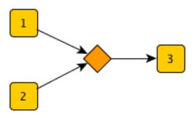
A *synchronization* pattern refers to a workflow in which the main thread waits for one or more concurrently-running tasks to complete before continuing. It is implemented by calling Core#wait\_for\_all with the futures that are returned from the activities that you want to synchronize:
