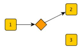
An *exclusive choice* pattern refers to a workflow in which the results of one activity are used to select one subsequent activity to run from a set of two or more activities. It is implemented by choosing the activity to run based on the value returned by a predicate function acting on a decision value:
