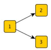
A *parallel split* pattern refers to a workflow in which one or more tasks are executed concurrently. It is implemented by calling activities asynchronously with GenericClient#send\_async:
