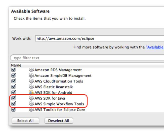
If you installed *all* of the available packages (by clicking the **AWS Toolkit for Eclipse** top-level node, or clicking **Select All**), both of these packages were automatically selected and installed for you.
