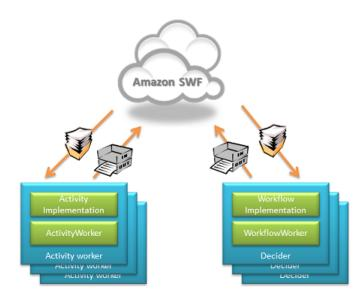
Moreover, each worker can be configured to process tasks on multiple threads. This means that the activity tasks of a workflow instance can run concurrently even if there is only one worker.
