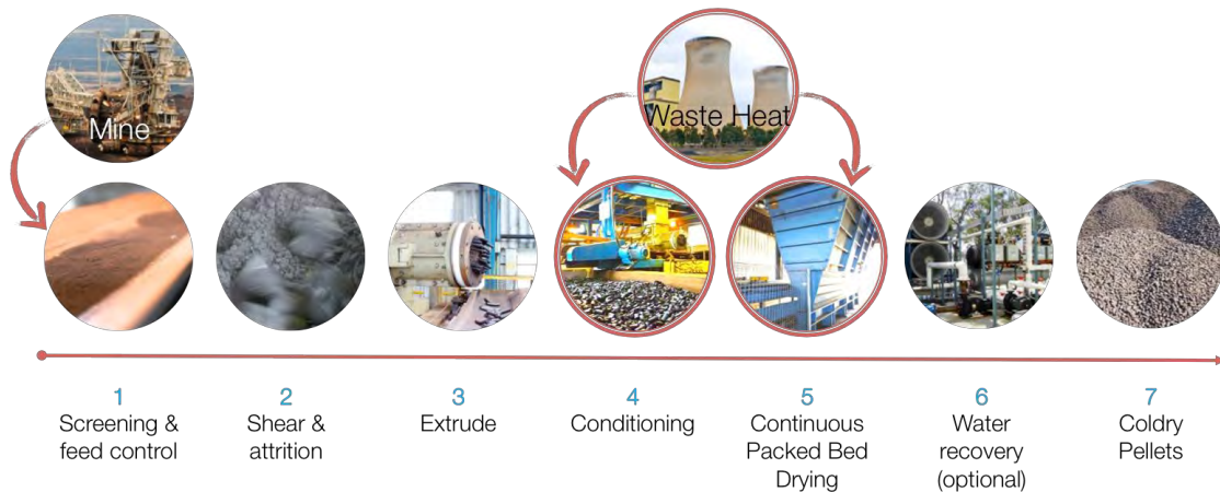
Figure 63: Coldry processing steps
