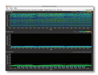
spectrum is not guaranteed on any certain frequencies. Previously, an off-the-shelf spectrum analyzer (which may cost upwards of \$10,000) was required to conduct a site survey or spectrum analysis at the installation site of the wireless equipment. Now integrated on all Ubiquiti Networks™ airMAX® M products, airView® provides powerful spectrum analyzer functionality, removing the need to rent or purchase additional equipment for doing site surveys.
