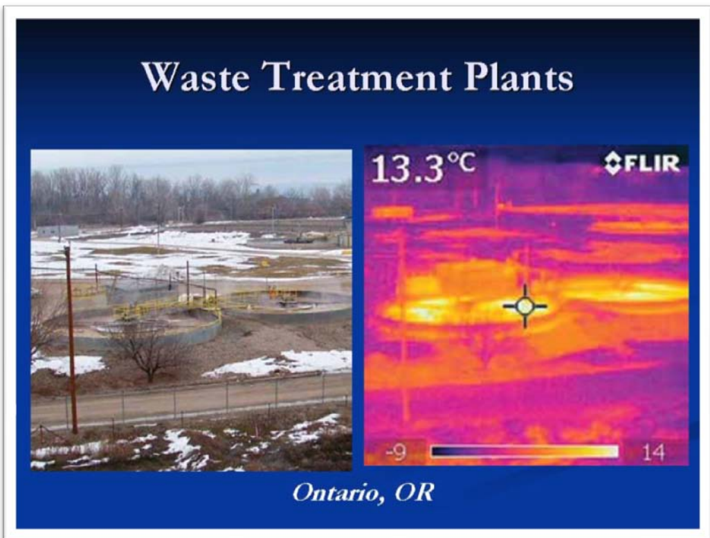
Numerous sensors are located at waste treatment plants. An infrared image of the scene shows the output of heat from the waste treatment beds right next to the sensor. (Photos by Anthony Watts, surfacestations.org .)
