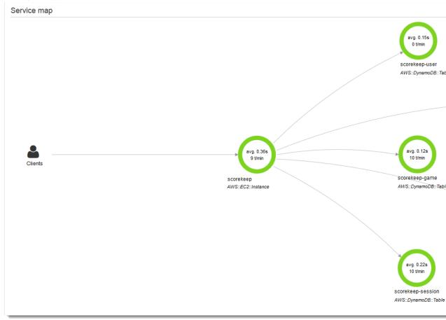
The service map shows the web app client, the API running in Elastic Beanstalk, the DynamoDB service, and each DynamoDB table that the application uses. Every request to the application, up to a configurable maximum number of requests per second, is traced as it hits the API, generates requests to downstream services, and completes.
