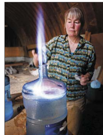
An Alberta homeowner ignites gas trapped in water from her well. A test showed strong similarities between the gas and drilling fluids used at a nearby gas well.
