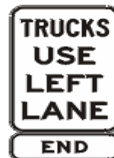
End trucks use left lane sign
